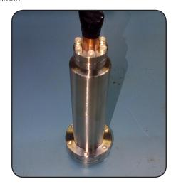
**CAUTION:** Do not remove the NEG from the transit case until you are ready to install it into your vacuum system. The NEG's performance is degraded through long term exposure to atmospheric conditions. Opening the NEG to a nitrogen environment is preferred but not required.
